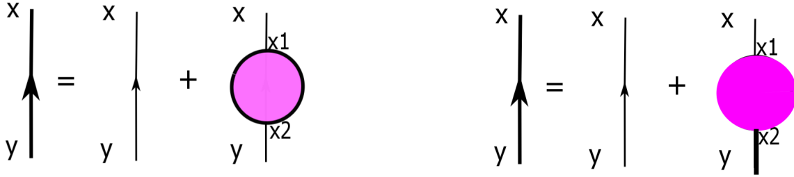
Figure 1.8: (Left) Feynman diagram for Dyson equation, where the pink circle stands for the (total) self-energy function. (Right) Feynman diagram for Dyson equation, where the pink circle stands for the proper self-energy function. The thin line is free Green's function, and the thick line is full Green's function.
